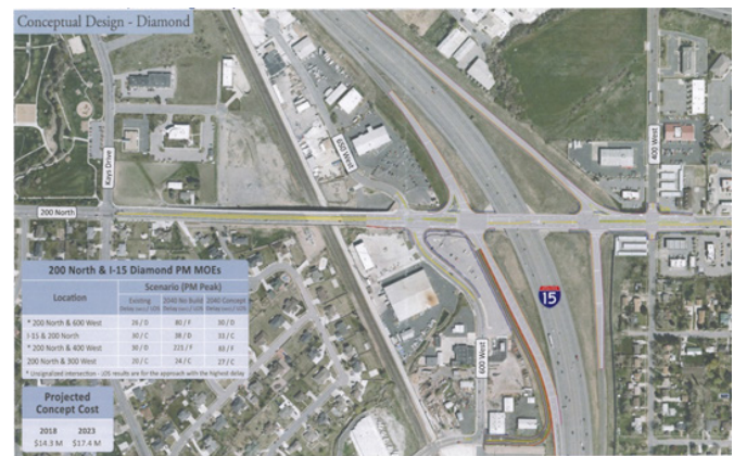
Concept developed by UDOT to increase mobility and safety at 200 North/I-15 interchange
