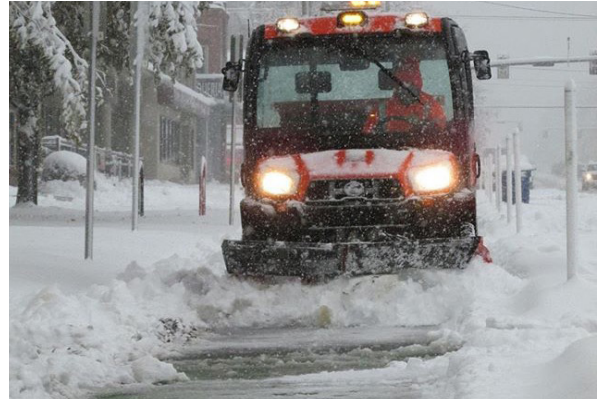
A small tractor with a narrow plow attached clears a separated bike lane during a winter snow storm in Salt Lake City (Photo: SLC Public Works)
